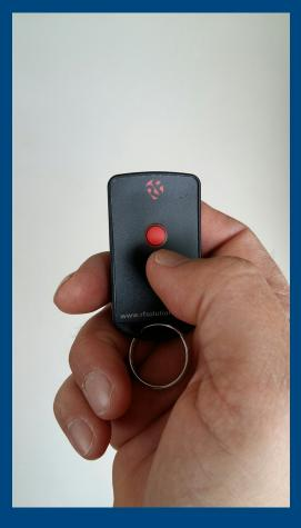
The NorFob is connected to the general I/O socket of the Norsonic sound level meters. Trigger conditions (start a measurement or start an audio recording) can be set on the Norsonic sound level meter.
