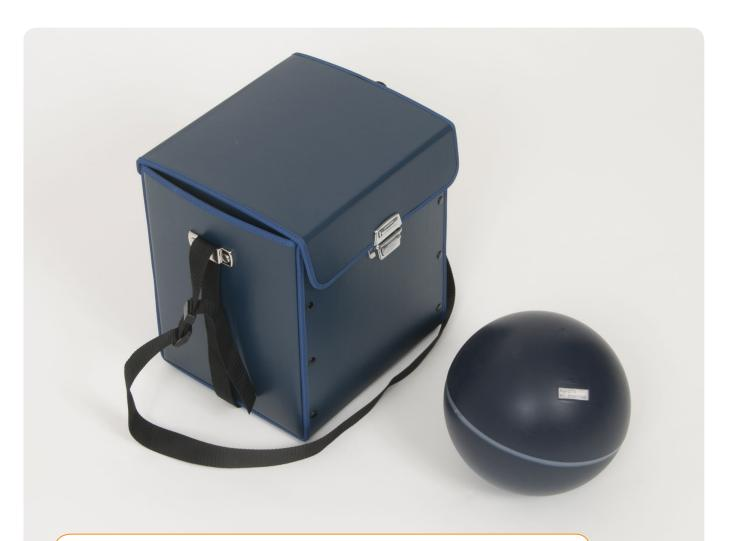
To be used as the "Rubber Ball " lower-frequency alternative to the Tapping Machine Excitation method in accordance with the ISO 16283-2 Appendix A.2 and the ISO 10140-5 Appendix F.2
